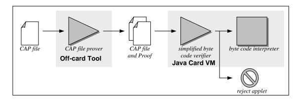
The "proof" generated is similar to the StackMap attribute used by the KVM, and contains the same kind of information. In our development, we add it in an additional component to the CAP file (for example COMPONENT\_Proof, or COMPONENT\_StackMap to follow the KVM naming convention).
